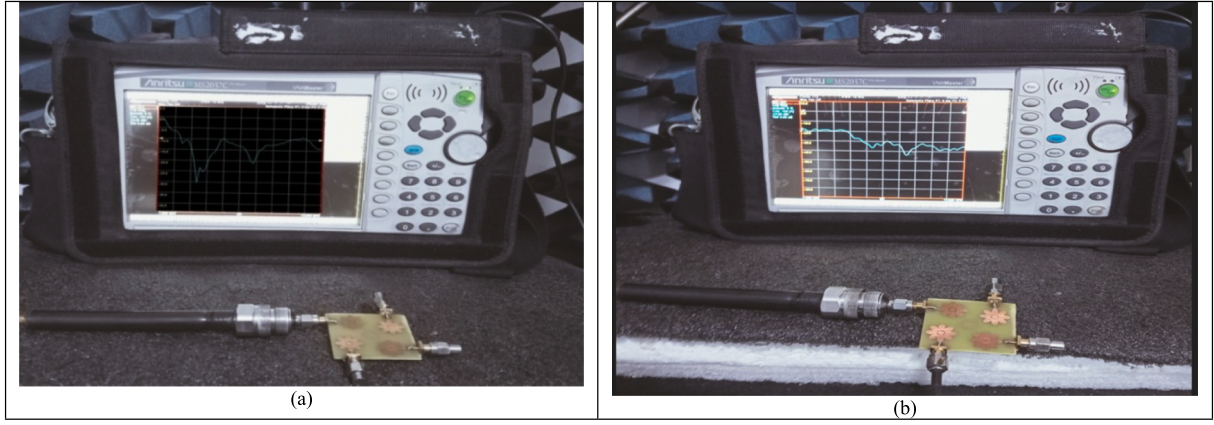
Fig. 10. Measurement of (a) return losses and (b) isolation.
