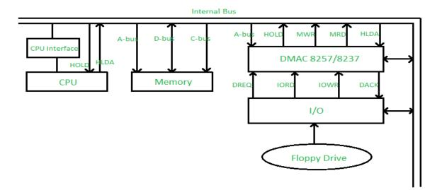
Suppose a floppy drive that is connected at input-output port wants to transfer data to memory, the following steps are performed:
